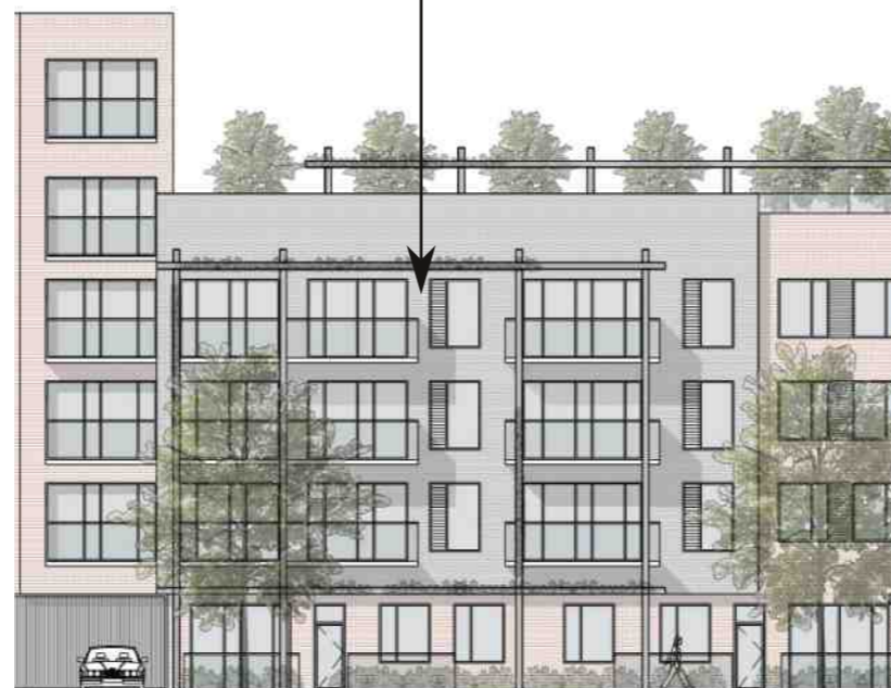
Block 5 West Elevation to Beltree Park Painted steel planted pergola structure at balconies With opaque glazed screens for privacy
